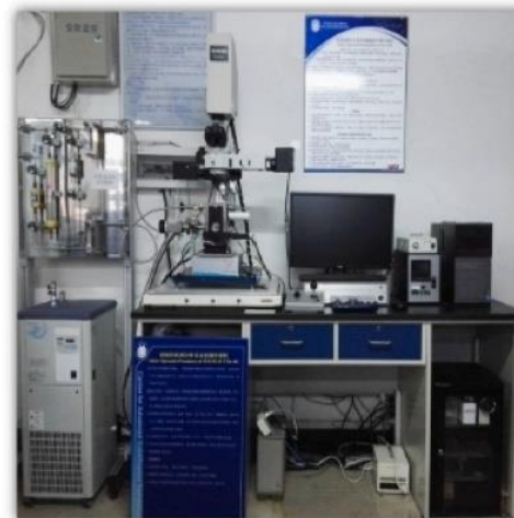
Fig. 22 High temperature confocal microscope
