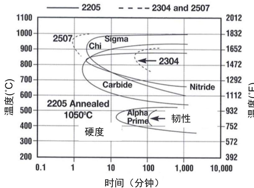
Isothermal precipitation kinetics of intermediates phases in duplex stainless steels
